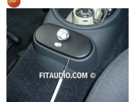
Start by un-clipping the gear gator surround and lifting this up, then remove the black cover at the back of the center console watching you don't loose the silver knob on the top (it pops off!).
