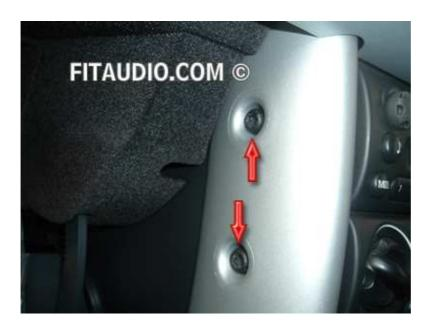
Now remove using your torx screwdriver set the two screws on each side of the main silver pillars
